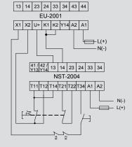
2. 2-channel operation connected to NST-2004
