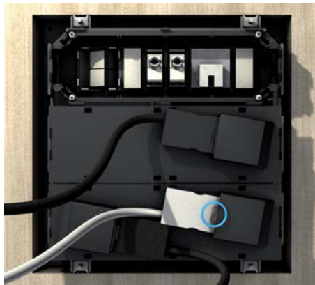
5 | Plug connector Self-locking and coded plug connectors facilitate faultless mounting with the device cup. To release, unlatch the grey spring catch with a turn screw.
