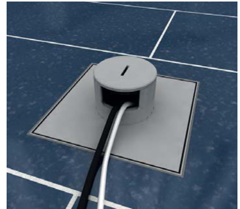
12 | Tube Insert rubber seal and tube cover. In case of wet maintenance floors, mount single tube outlet and tube. Comply with potential equalization.
