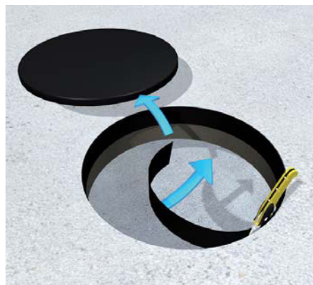
5 | Cut out opening After the screed has hardened remove the overlapping lid and sidewalls neatly.
