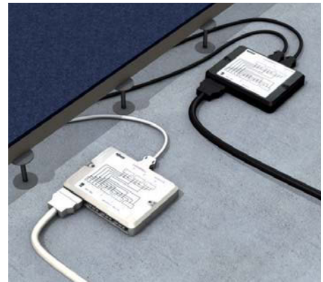
6 | Underfloor distributor Insert the plug of the 3-pole connecting line in one of the six output sockets of the distributor and complete with 5-pole input.
