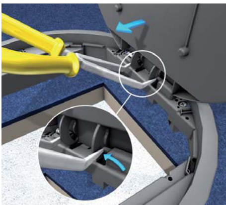
4 | Hinged cover removal Press hinge together using pliers until the lugs snap out of the frame. Remove cover towards the front.
