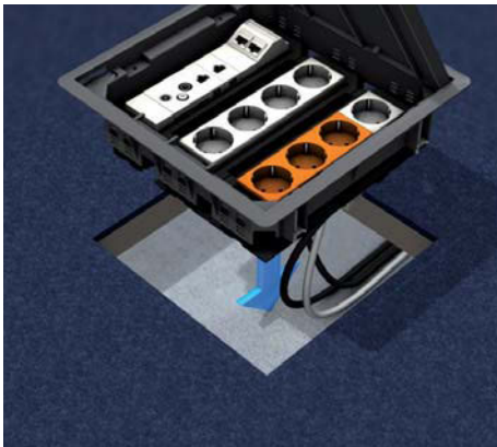
4 | Installation unit Place the complete installation unit with the device cups from the top into the existing floor opening and fixate in the floor with claws.
