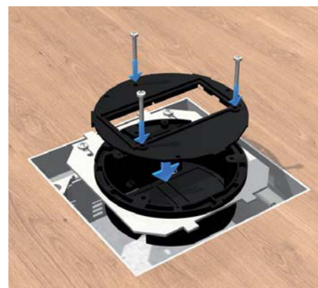
6 | Cover plate Fix the cover plate onto the device cup with screws.
