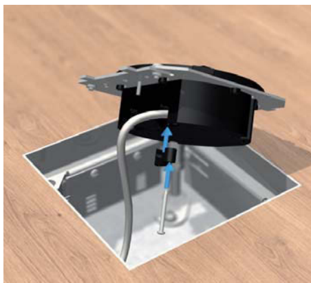
8 | Device cup Place the device cup into the plate, insert the ducts into strain relief and screw in the fixing bolt.
