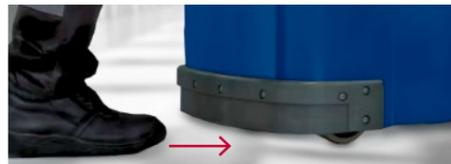
2 Vehicle equipped with foot protection switch. After collision and stop, the vehicle reverses.
